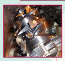
Cutting plates are fixed on holders welded on the segment. Turning and replacement of the cutting plates are easy and short.
